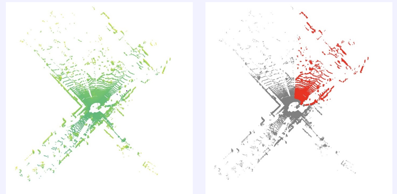
Full LiDAR point cloud Camera-FOV region marked in red In SemanticKITTI, the LiDAR observes the full surrounding scene, while the camera only covers a limited forward-facing region. Our approach leverages shared 3D parameters learned under 2D supervision, allowing out-of-FOV points to benefit indirectly from cross-modal alignment.
